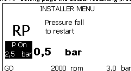
Figure 18.1: Setting the restart pressure (1)
