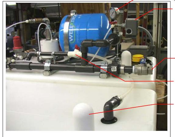
1" FIP connection for pressure discharge to shower. Not shown is bypass on other side of wall
