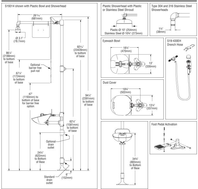
All dimensions assume standard thread engagement. Variations in manufacturing allow for  $+/- \frac{1}{3}$ "(3mm) per threaded joint. To find the tolerance of a dimension, add the number of thread joints across the length of the dimension and multiply it by  $\frac{1}{3}$ " (3mm).
