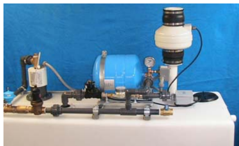
System with a Spray Boom and exhaust fan wired to run during fill cycles.
